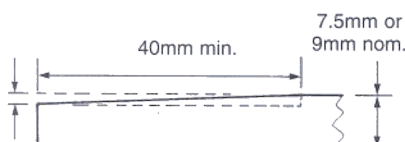
Fig. 7 SITE-GROUND RECESSED-EDGE DETAIL
